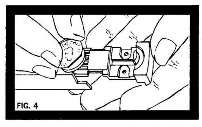
The length of spacer is not critical unless your cartridge is unusualy long and will not fit within the head. In that case, select a pair of spacers that will permit the cartridge to clear the
