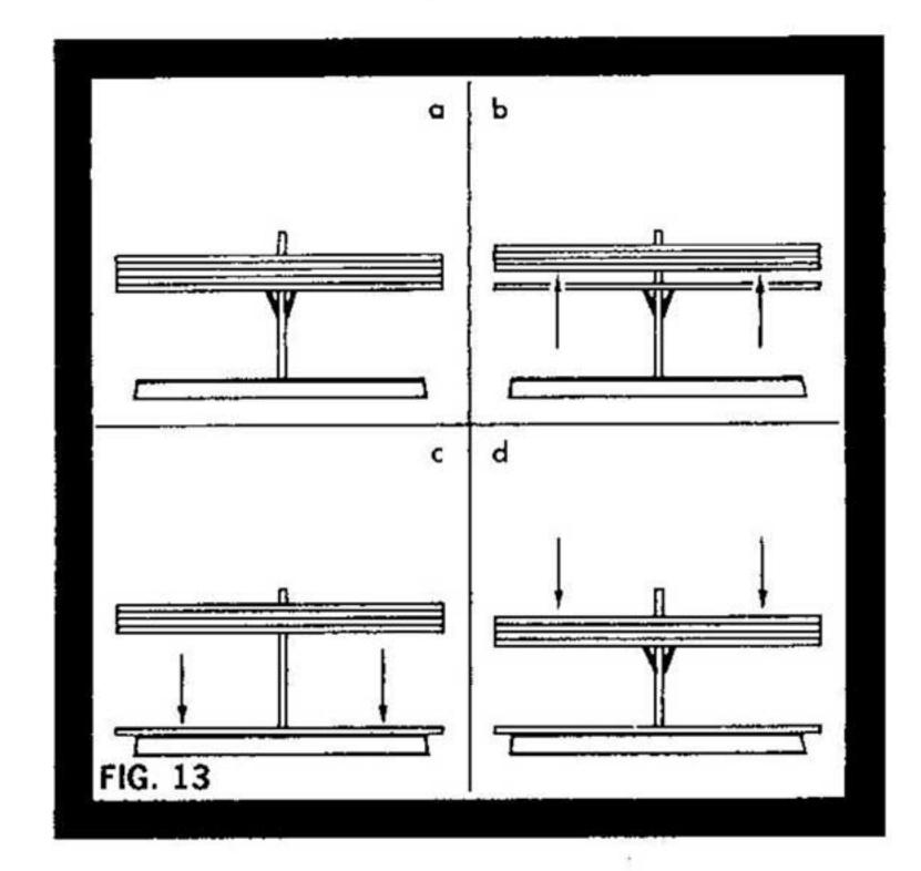
The entire stack rests upon a three-pronged platform (fig. 13a). When the slide switch is pushed to START, the weight of the entire stack is lifted off the bottom record (b), which is then released to descend to the turntable (c). The stack now lowers (d) to await the next change cycle.
