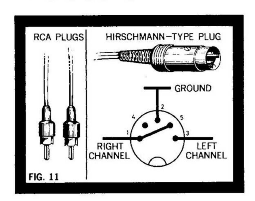
for left channel, and the yellow cable for right channel. The Hirschmann-type plug, supplied with some models, is also illustrated, along with its channel connection schematic. Connect the appropriate plug according to the directions supplied with your amplifier(s) ... or with other high quality audio equipment designed for use with component record players.
