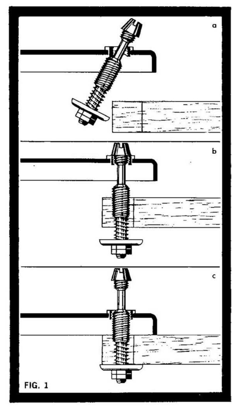
the right and rear to provide for the tonearm's unusually short overhang.) Here's how it's done. Hold the chassis above the base so that the three spring-mounted footings will fit into their cut-outs. As you lower the chassis, tilt the spring screws (fig. 1a) to let them slip past the special notches. Then turn each screw clockwise until it is firmly seated into the top of the chassis (fig. 1b). To remove the Dual simply reverse the procedure.
