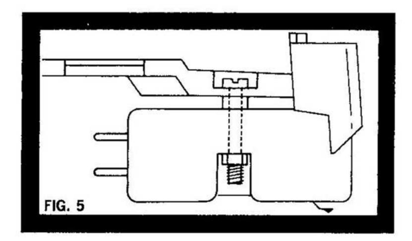
front of the head. Note in fig. 5 that the head of the screw should be against the holder, not the nut.
