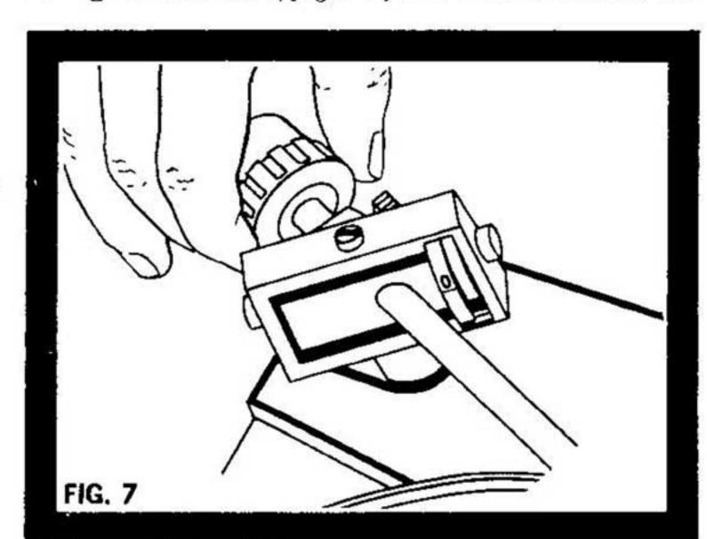
the tonearm needs to be lightened, rotate the weight clockwise . . . and vice versa. When the tonearm is in perfect horizontal balance, apply the desired stylus force (as recommended by the manufacturer of your cartridge) by turning the stylus force scale to the number indicated (fig. 8).
